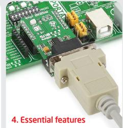
The RS232 DB9 port (9 pins) and the MAX3232 IC constitute a serial communications connector. RS232 is mostly used for industrial machines, networking equipment and scientific instruments, as well as for computer peripherals. The board features two jumper positions to connect RTS (J2) and CTS (J3) lines to the target board (zero-ohm SMD jumpers not provided in the package).
