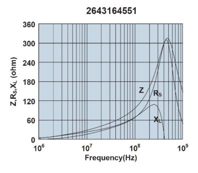
Impedance, reactance, and resistance vs. frequency.
