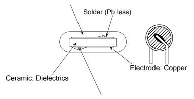
Lead wire: CP wire (Tin plated copper covers steel wire, Pb less)
