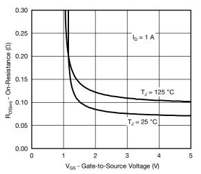
**On-Resistance vs. Gate-to-Source Voltage**
