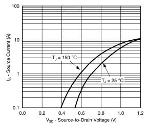
Source-Drain Diode Forward Voltage
