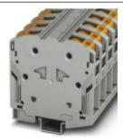
High-current terminal block, Connection method: Push-in connection, Cross section: 25 mm<sup>2</sup> - 95 mm<sup>2</sup>, AWG: 4 - 3/0, Width: 25 mm, Color: gray, Mounting type: NS 35/15
