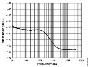
Figure 8. Phase Noise, PLL1, OUT0 LVPECL, 156.25 MHz Integer-N Mode  $(f_{XTAL} = 25 \text{ MHz}, Na = 100, V0 = 4, D0 = 4)$
