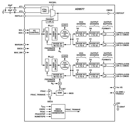
Figure 32. Detailed Block Diagram
