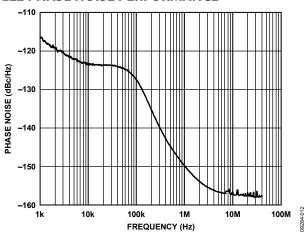
Figure 12. Phase Noise, PLL2, OUT2 LVPECL, 100 MHz, Integer-N Mode  $(f_{XTAL} = 25 \text{ MHz}, Nb = 100, V2 = 5, D2 = 5)$
