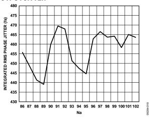
Figure 18. Typical Integrated Random Phase Jitter in fs rms for PLL1 and OUTOP LVPECL as Feedback Divider Value Na Swept ( $f_{XTAL} = 25$  MHz, VO = 5, DO = 5)
