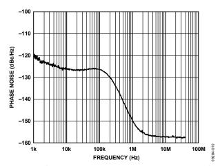
Figure 10. Phase Noise, PLL1, OUT0 LVPECL, 125 MHz, Integer-N Mode  $(f_{XTAL} = 25 \text{ MHz}, Na = 100, V0 = 4, D0 = 5)$
