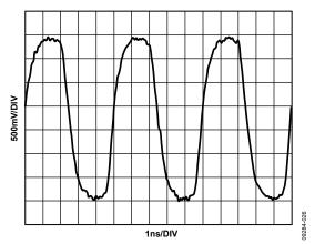
Figure 22. Typical CMOS Output Trace, 200MHz
