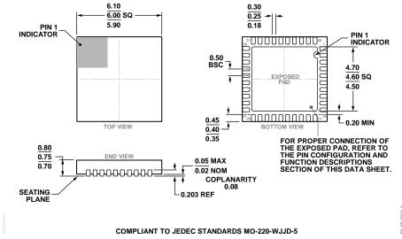
Figure 51. 40-Lead Lead Frame Chip Scale Package [LFCSP\_WQ] 6 mm × 6 mm Body, Very Very Thin Quad (CP-40-7) Dimensions shown in millimeters
