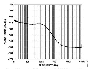
Figure 11. Phase Noise, PLL1, OUT0 LVPECL, 625 MHz, Integer-N Mode  $(f_{XTAL} = 25 \text{ MHz}, Na = 100, V0 = 2, D0 = 2)$
