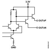
Figure 37. LVPECL Outputs Simplified Equivalent Circuit
