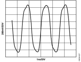
Figure 23. Typical LVPECL Differential Output Trace, 625 MHz
