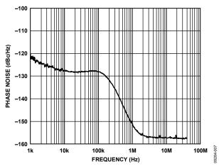
Figure 7. Phase Noise, PLL1, OUT0 LVPECL, 106.25 MHz, Integer-N Mode  $(f_{XTAL} = 25 \text{ MHz}, Na = 102, V0 = 4, D0 = 6)$
