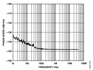
Figure 6. Phase Noise, REFOUT Output, 25 MHz ( $f_{XTAL} = 25$  MHz)
