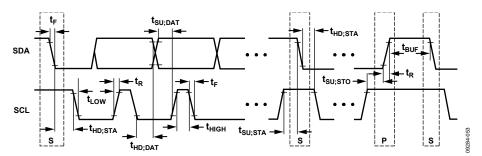
Figure 48. I<sup>2</sup>C Port Timing Diagram
