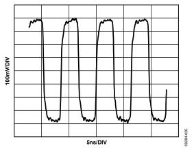
Figure 21. Typical LVDS Differential Output Trace, 156.25 MHz
