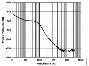
Figure 14. Phase Noise, PLL2, OUT2 LVPECL, 155.52 MHz, Fractional-N Mode (f<sub>XTAL</sub> = 25 MHz, Nb = 99, FRAC = 333, MOD = 625, V2 = 2, D2 = 8), Spurs Disabled
