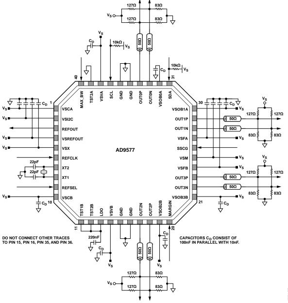
Figure 50. Typical LVPECL Application Circuit
