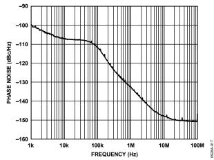
Figure 17. Phase Noise, PLL2, OUT2 LVPECL, 622.08 MHz, Fractional-N Mode  $(f_{XTAL}=25 \text{ MHz}, \text{Nb}=99, \text{FRAC}=333, \text{MOD}=625, \text{V2}=2, \text{D2}=2)$ , Spurs Disabled
