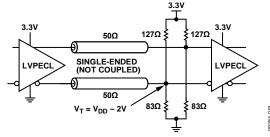
Figure 39. LVPECL DC-Coupled Termination
