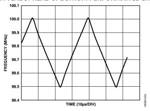
Figure 29. Typical Spread Spectrum Frequency Modulation Profile OUT2, Nb = 96, FRAC = 0, MOD = 1000, CkDiv = 7, NumSteps = 59, FracStep = -8,  $f_{OUT} = 100$  MHz with -0.5% Downspread at 30.2 kHz,  $MAX_BW$  set to 0
