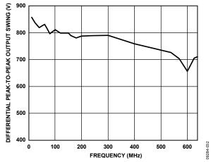
Figure 28. LVDS Differential, Peak-to-Peak Output Swing vs. Frequency
