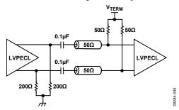
Figure 41. LVPECL AC-Coupled Termination
