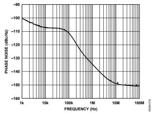
Figure 16. Phase Noise, PLL2, OUT2 LVPECL, 625 MHz, Integer-N Mode  $(f_{XTAL} = 25 \text{ MHz}, Nb = 100, V2 = 2, D2 = 2)$
