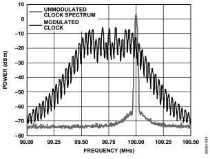
Figure 30. Typical Nonspread and Spread Spectrum Power Spectra, OUT2, Nb = 96, FRAC = 0, MOD = 1000, CkDiv = 7, NumSteps = 59, FracStep = -8,  $f_{OUT} = 100$  MHz with -0.5% Downspread at 30.2 kHz,  $MAX_BW$  set to 0, First Harmonic Shown, Spectrum Analyzer Resolution Bandwidth = 10 kHz,  $Max_BW$  Maximum Hold On
