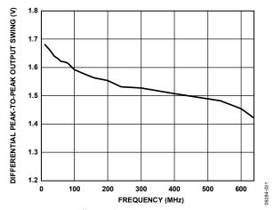
Figure 27. LVPECL Differential, Peak-to-Peak Output Swing vs. Frequency
