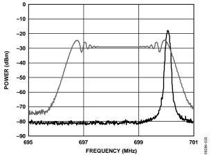
Figure 31. Typical Nonspread and Spread Spectrum Power Spectra, OUT2, Nb = 96, FRAC = 0, MOD = 1000, CkDiv = 7, NumSteps = 59, FracStep = -8,  $f_{OUT} = 100$  MHz with -0.5% Downspread at 30.2 kHz,  $MAX_BW$  set to 0, Seventh Harmonic Shown, Spectrum Analyzer Resolution Bandwidth = 120 kHz, Maximum Hold On
