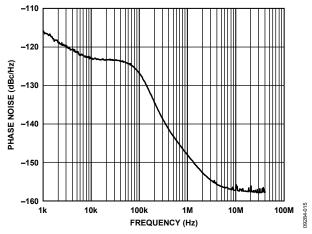
Figure 15. Phase Noise, PLL2, OUT2 LVPECL, 106.25 MHz, Integer-N Mode  $(f_{XTAL} = 25 \text{ MHz}, \text{Nb} = 102, \text{V2} = 4, \text{D2} = 6)$
