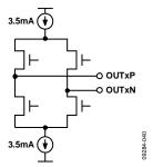
Figure 36. LVDS Outputs Simplified Equivalent Circuit
