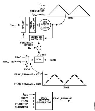
Figure 43. Spread Spectrum Clock Generator with Triangular Wave Modulation, f<sub>PFD</sub> = 25 MHz
