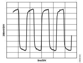
Figure 20 Typical LVPECL Differential Output Trace, 156.25 MHz
