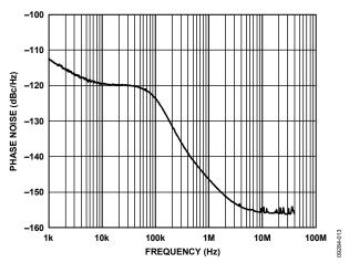
Figure 13. Phase Noise, PLL2, OUT2 LVPECL, 156.25 MHz, Integer-N Mode  $(f_{XTAL} = 25 \text{ MHz}, \text{Nb} = 100, \text{V2} = 4, \text{D2} = 4)$
