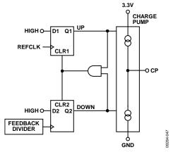
Figure 42. PFD Circuit Showing Simplified Charge Pump
