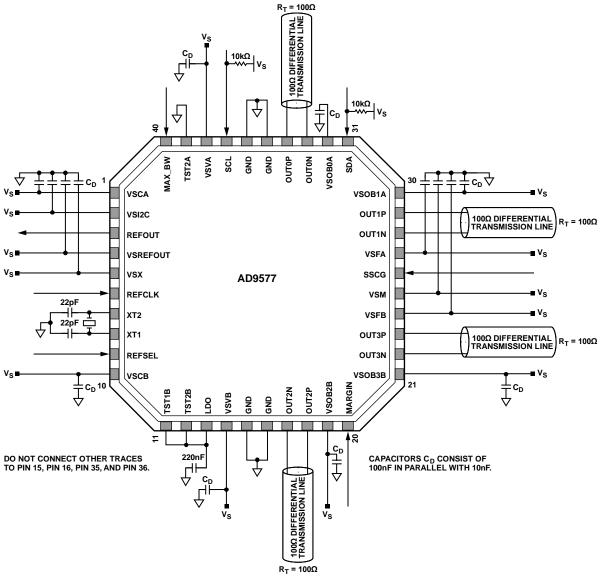
Figure 49. Typical LVDS Application Circuit
