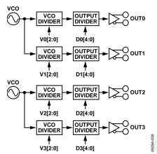
Figure 35. Output Channel Divider Signal Path
