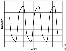
Figure 24. Typical LVDS Differential Output Trace, 625 MHz
