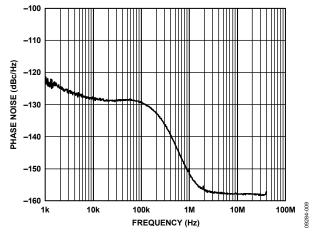
Figure 9. Phase Noise, PLL1, OUT0 LVPECL, 100 MHz, Integer-N Mode  $(f_{XTAL} = 25 \text{ MHz}, Na = 100, V0 = 5, D0 = 5)$
