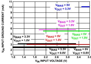
FIGURE 14. INPUT GROUND CURRENT vs  $V_{IN}$  and  $V_{OUT}$
