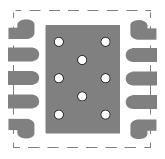
FIGURE 39. PCB VIA PATTERN
