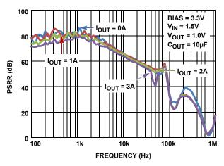
FIGURE 30.  $V_{\mbox{\scriptsize IN}}$  PSRR vs FREQUENCY FOR VARIOUS LOAD CURRENTS
