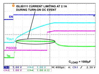
FIGURE 21. ISL80111 ENABLED INTO OVERCURRENT
