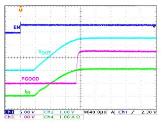
FIGURE 19. ENABLE START-UP WITH PGOOD
