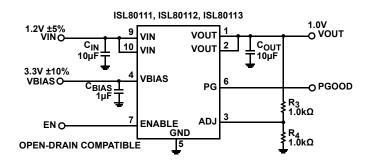
FIGURE 1. TYPICAL APPLICATION SCHEMATIC
