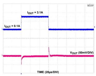
FIGURE 27. 3A LOAD TRANSIENT RESPONSE
