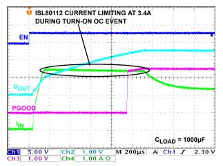
FIGURE 22. ISL80112 ENABLED INTO OVERCURRENT
