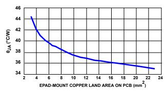
FIGURE 38. 3mmx3mm-10 PIN DFN ON 4-LAYER PCB WITH THERMAL VIAS  $\theta_{JA}$  vs EPAD-MOUNT COPPER LAND **AREA ON PCB**
