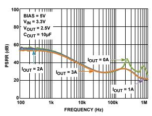
FIGURE 29. BIAS PSRR vs FREQUENCY FOR VARIOUS LOAD **CURRENTS**
