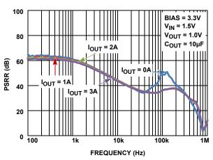
FIGURE 31.  $V_{\mbox{\footnotesize BIAS}}$  PSRR vs FREQUENCY FOR VARIOUS LOAD
