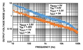
FIGURE 37. OUTPUT NOISE SPECTRAL DENSITY
