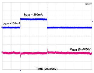
FIGURE 24. 100mA LOAD TRANSIENT RESPONSE
