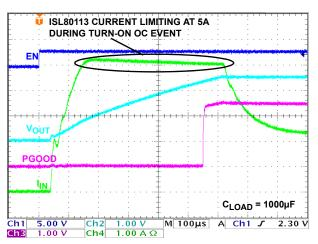
FIGURE 23. ISL80113 ENABLED INTO OVERCURRENT
