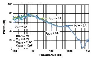
FIGURE 3. VIN PSRR vs LOAD CURRENT (ISL80113)
