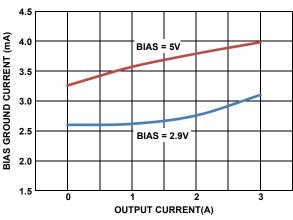
FIGURE 13. BIAS GROUND CURRENT vs LOAD CURRENT
