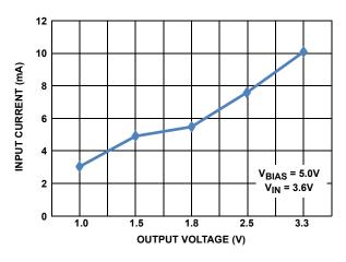
FIGURE 18.  $V_{IN} I_Q vs VOUT VOLTAGE$
