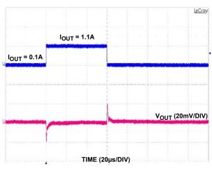
FIGURE 25. 1A LOAD TRANSIENT RESPONSE
