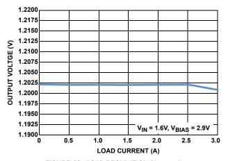
FIGURE 10. LOAD REGULATION,  $V_{OUT}$  vs  $I_{OUT}$
