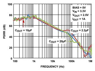
FIGURE 33. VIN PSRR vs FREQUENCY FOR VARIOUS COUT
