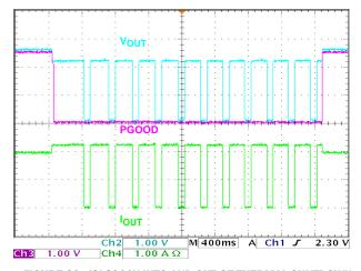
FIGURE 20. ISL8011X INTO AND OUT OF THERMAL SHUTDOWN
