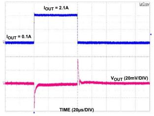
FIGURE 26. 2A LOAD TRANSIENT RESPONSE
