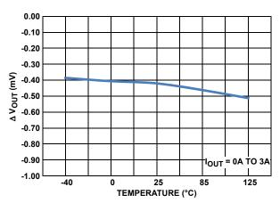
FIGURE 9. LOAD REGULATION vs TEMPERATURE
