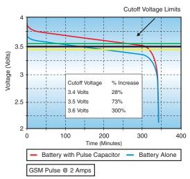
Figure 6a. Li-ION Battery at +25°C
