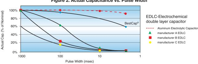
Figure 2. Actual Capacitance vs. Pulse Width
