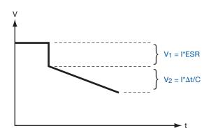
It is assumed that during the pulse, 0.5A is delivered by the battery and 1.5A by the capacitor.
