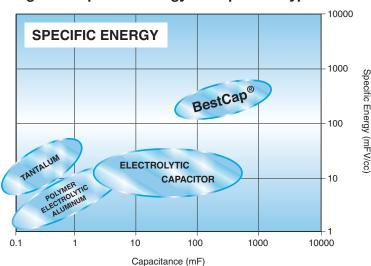
Figure 1. Specific Energy of Capacitor Types
