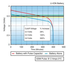
Figure 6b. Li-ION Battery at +0°C
