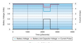
Figure 5. GSM Pulse
