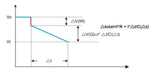
Figure 4. Voltage-time relation of capacitor unit
