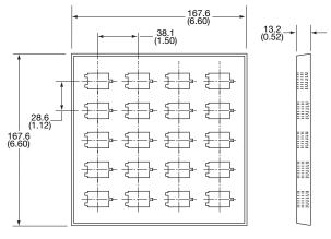
This specification applies when our electrochemical supercapacitors are packed using a 165mm by 165mm container. The parts are held in place by a 166mm by 166mm lid.
