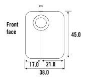
This innovative design provides a high accuracy, non-invasive, flow measurement device at a fraction of the cost of other current non-invasive systems. The unique measurement technique automatically compensates for viscosity and temperature variations. The measurement of flow is by ultrasonic transit time in-line cell.
